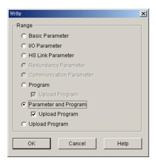
After saving *High Speed Link* parameter written by the user in GMWIN project file and connecting to PLC through 'online connect' of GMWIN basic menu, select 'write' and the window 'write' appears as above. If you select '*High Speed Link* parameter' or 'parameter and program' from the above menu and download the selected parameter, the corresponding contents shall be downloaded.
