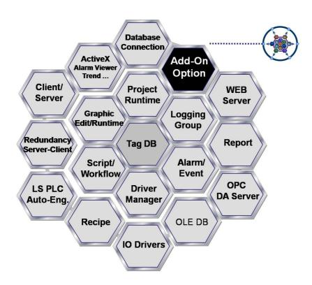
InfoU software is made up of the components as seen in the figure above and the structure of this software allows the user to add other various components to its basic ones and those newly added components are internally connected through data communication and API to act dependently on each other.
